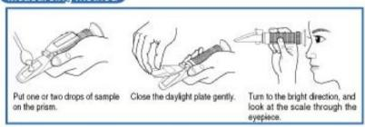
Refractive index of a solution varies according to the its concentration. Hence, its concentration is obtained from its refractive index. The refractive index of blood serum or plasma depends mainly upon its protein concentration, as proteins are one of the major constituents.
