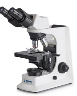
trinocular and phase contrast model. KERN OBL-1 also available with EPI fluorescence illumination unit on request
