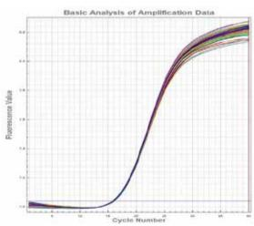
Simultaneous scanning of the six-channel shows that the standard deviation of the Ct value of the FAM channel is <0.07. No fluorescence signal in other channels.
