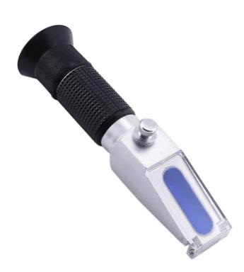
Our new item is designed for clinical usage and intended for both Veterinary and Human. This unit provides quick and accurate indication of vital fluids levels. It has triple scale that gives Urine Specific Gravity(SG), Total Serum Protein(SP) and Refractive Index (RI). It's FULLY EQUIPPED with ATC that automatically adjust itself to correct temperature discrepancies during use. Capable of measuring with high accuracy and provides precise results.
