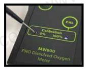
The MW600 PRO calibrates easily in 2 points (at 100% saturated air and in 0 Oxygen solution) and has Automatic Temperature Compensation which guarantees highest accuracy.
